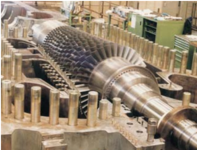
Mixed Refrigerant Compressor for LNG Plant
