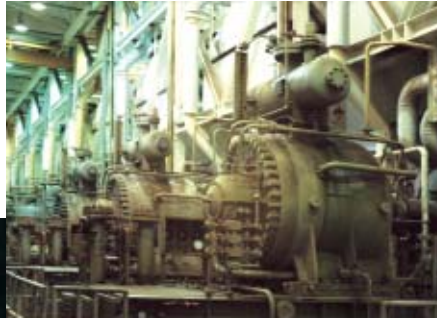
The PCL 802 centrifugal compressor boosting natural gas on board the main Ekofisk platform
