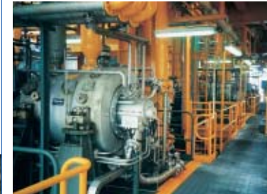
BCL 406/B + BCL 305/C driven by MS5002 Gas Turbine installed on Nkossa platform - Congo
