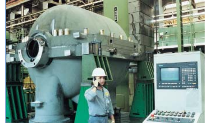
2MCL Horizontally split compressor being machined
